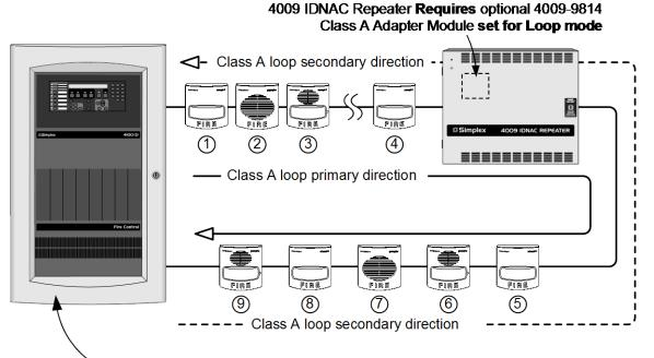
Simplex Fire Alarm Control Panel with IDNAC SLC; **requires** optional Dual Class A IDNAC Isolator (DCAI), refer to individual panel documentation for details (4100ES with EPS shown for reference)
